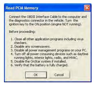
Before proceeding, connect the RS-232 to OBDII converter interface to the Comm port on your PC. If your PC has more than one Comm port, make sure you connect the converter to the com port that you specified on the Comm Port Setup screen.
