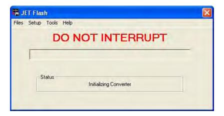
The progress meter shows the progress on the programming as it proceeds and the Status window describes what part of the process in currently underway. Depending on the PC you are using, the programming will usually take a minute or two.
