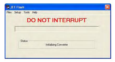
The progress meter shows the progress on the reading of the PCM as it proceeds and the Status window describes what part of the process is currently underway. Depending on the type of vehicle and the PC you are using, the read will usually take about four minutes.
